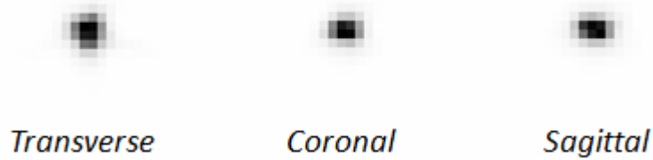
Figure 11: Focused reconstructed point source in transverse, coronal and sagittal slice view
